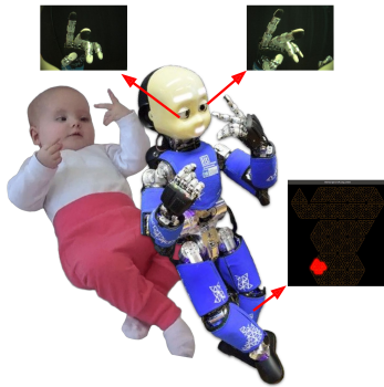
Fig. 3: Motion retargeting – infant to humanoids. The estimated infant pose or motion is retargeted onto a target robot or simulator platform. Here, the target is the iCub humanoid robot. The sensors of the robot can be used to emulate the first-person sensory experiences of the infant—vision and touch in this case. See (López et al., 2026) for details.
