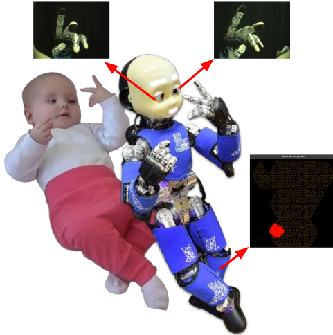
Fig. 3: Motion retargeting – infant to humanoid. The estimated infant pose or motion is retargeted onto a target robot or simulator platform. Here, the target is the iCub humanoid robot. The sensors of the robot can be used to emulate the first-person sensory experiences of the infant—vision and touch in this case. See (Lopez et al., 2026) for details.
